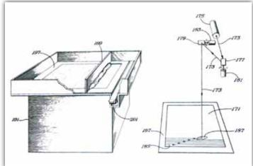
Early additive manufacturing laser-based powder processes of Ciraud<sup>10</sup> and Housholder<sup>12</sup>.
