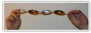
Roll plated and twisted band made from aluminum and copper.
