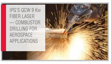
To be precise, "the typical jet engine has upwards of 3 million (transpiration cooling) holes that are percussion drilled," noted Bill Shiner, vice president of industrial markets for IPG. "With fiber lasers, we're getting better hole quality and better consistency, and we're drilling up to 50 to 100 holes per second."
