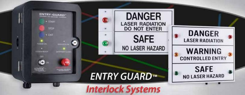
Entry-Guard™ is a Safety Interlock System (SIS) that provides a failsafe Access Control System (ACS). Its primary function is to ensure that unauthorized personnel are prohibited from areas where laser radiation may be present. When the power to the controller is interrupted, critical outputs, such as door magnetic locks and laser interlocks, revert to a safe state: magnetic locks off, interlocks open.
