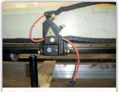
Figure 3. Air pump setup on laser machine
