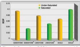
Figure 6. Comparison ROP between saturated & unsaturated samples
