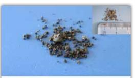
Figure 2: Laser drilling cutting (Mag. 12X)
