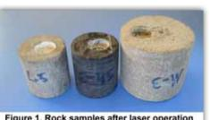
Figure 1. Rock samples after laser operation from left to right: Limestone, Shale, and Sandstone
