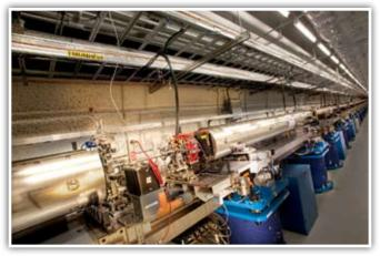
Only 12 of a total 33 LCLS undulator magnets (silvertone oblongs) were needed to create the first pulses of laser light. (Photo: Brad Plummer)
