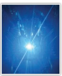
Hybrid welding in action using a CO, laser for a shipbuilding application
