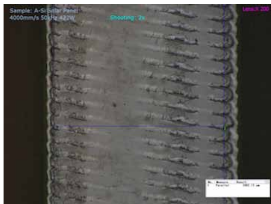
Fig. 2: Microscope image of the processed zone. Laser wavelength 1064 nm.
