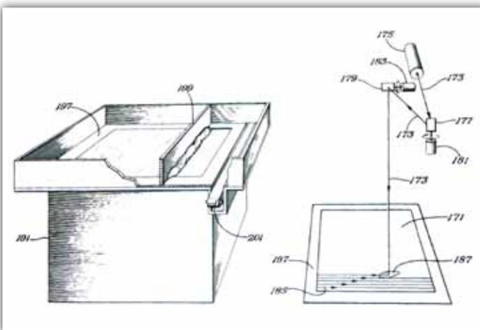
Early additive manufacturing laser-based powder processes of Ciraud<sup>10</sup> and Housholder<sup>12</sup>.
