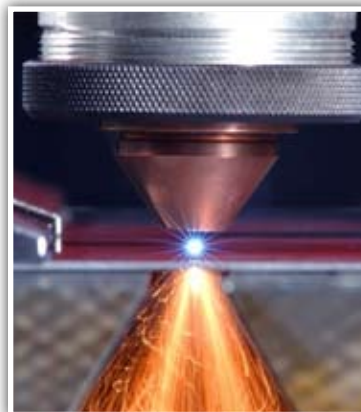
Figure 4: High-speed cutting of 1.2 mm car body steel.
