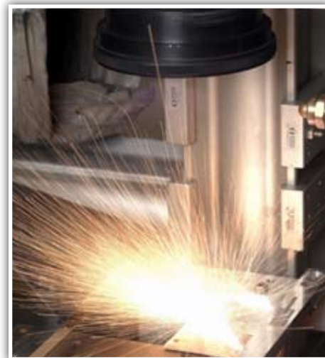
Figure 5: Remote cutting of 0.5 mm stainless steel.
