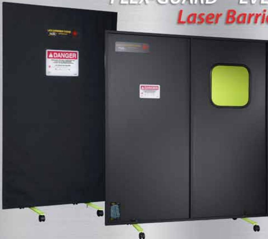
Flex-Guard™ heavy duty matte finish fabric is ideal for blocking diffuse and low power laser radiation. Durable and flame retardant materials are suspended from ceiling- or floor-mounted coated black steel track engineered for low-friction operation. Virtually any configuration is possible using curves, by-pass rollers and other accessories. Each system is rated up to 200W/cm<sup>2</sup> for 100 seconds and is available in stock and custom sizes.
