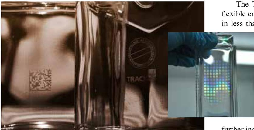
Examples of internal glass marking using ultrafast lasers.
