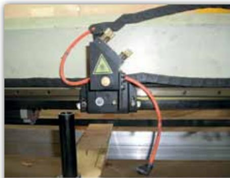
Figure 3. Air pump setup on laser machine
