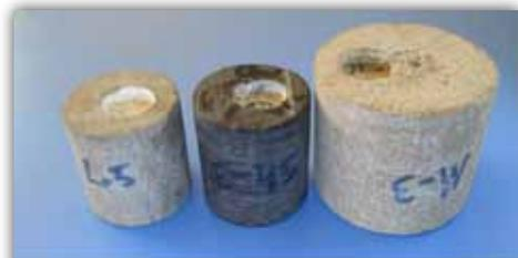
Figure 1. Rock samples after laser operation from left to right: Limestone, Shale, and Sandstone
