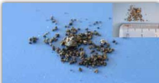
Figure 2: Laser drilling cutting (Mag. 12X)
