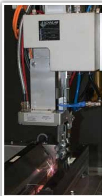
**Laser beam welding of Al-Cu compounds (process).**
