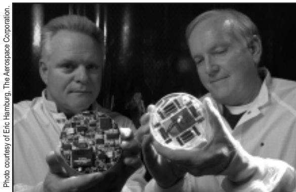
Lee Steffeney (left) and Bill Hansen of The Aerospace Corporation display segments of co-orbiting satellite assistant glass-ceramic propulsion modules with integrated inertial measurement unit.
